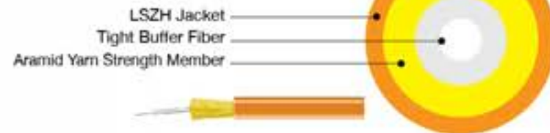
Simplex Optical Fiber Cable
